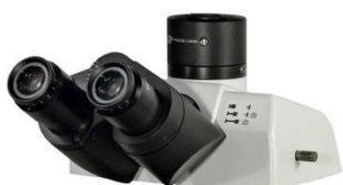
Low profile 20 degree fixed Eye tube ) with integrated Photo Port. User selectable 3 way light distribution: 100% visual \ 100% photo \ 20%vis-89% photo split
